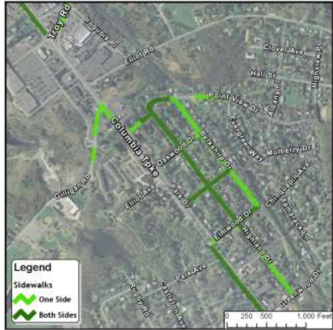
Columbia Turnpike Sidewalk Gaps: This is the largest gap in sidewalks along Columbia Turnpike, at over 3,000 feet in length, extending south from the intersection with Route 4 to Elmwood Drive. The residential neighborhood centered on Highland Drive, however, has an abundance of sidewalks. (Existing sidewalk locations shown in green.)
